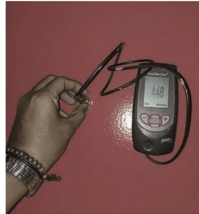
Gambar 12. Inspeksi *Dry Film Thickness*
