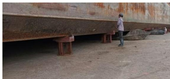
**Gambar 2.** *Scraping* Lambung Kapal
