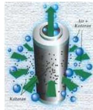
Gambar 5. Cara kerja *cartridge filter*
