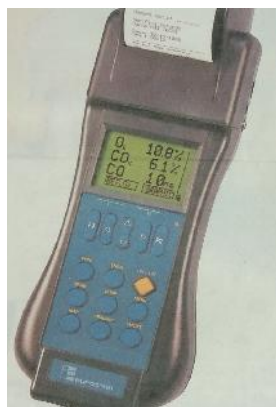
Gambar 4. GreenLine 4000 Gas Analyser
