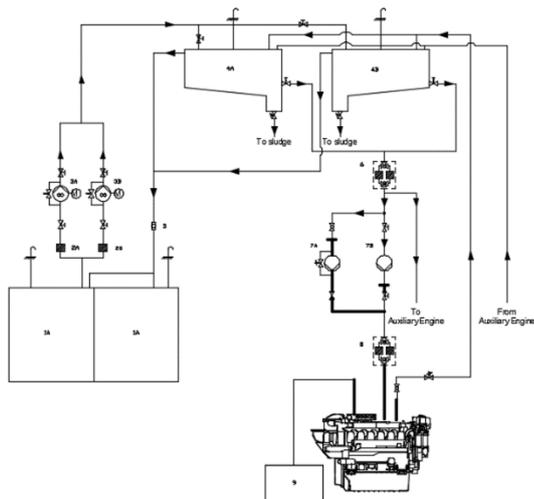
**Gambar 4.** Piping Diagram Fuel Oil
